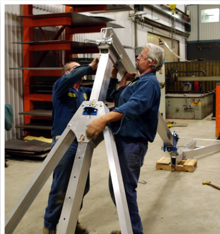
Aluminum gantry crane when folded for storage.
