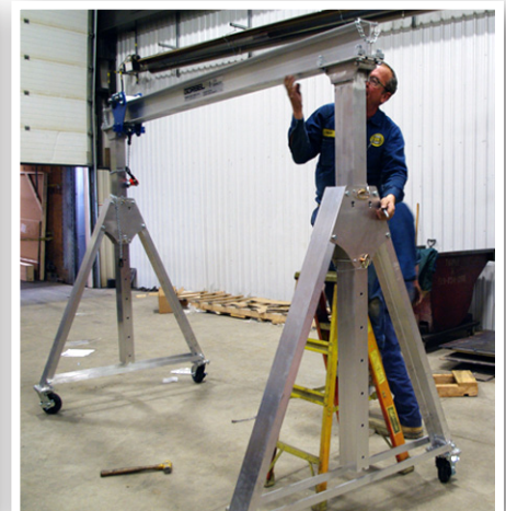
Aluminum gantry crane when folded for storage.
